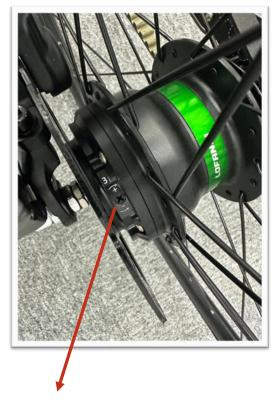
3rd gear adjustment screw Adjust first!
